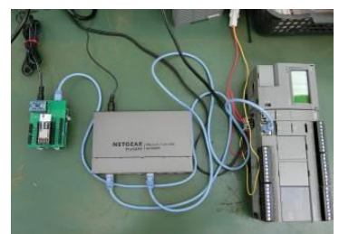
図4. PLC (Programmable Logic Controller)
